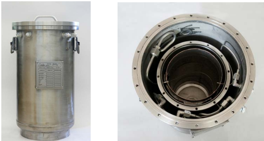
Figure 8. The transportable chamber for the calibration of AWS made at INRiM.
