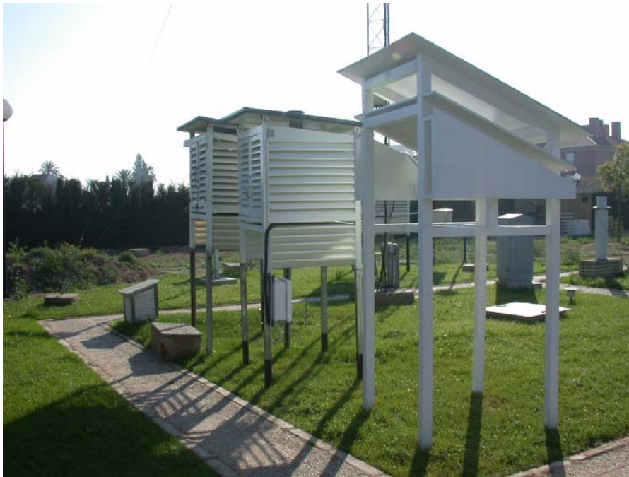
Figure 3. Picture showing the reproduction of the old Montsouris stand and the new Stevenson screen as replicated in the Meteorological Garden of Murcia (INM, Spain). Dual temperature observations are taken with identical sensors sheltered in a Stevenson screen (back) and in a Montsouris stand (in front). Courtesy of the project SCREEN
